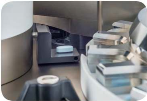
Precise tablet positioning (patented stamp)
